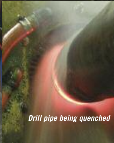
Inertia weld pre heating prior to quenching
